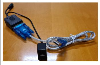
Each adapter can connect one DEC keyboard to one **vtXterm** graphical workstation.
