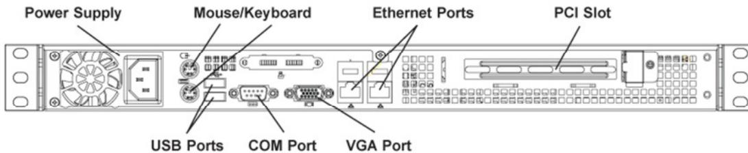
The external USB ports support the vtAlpha / vtVAX license key. Three additional USB ports are available inside the unit.
