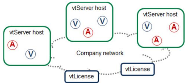
Each vtServer host may run one or more vtAlpha and vtVAX in-stances simultaneously. These instances may be either production or 'disaster recovery' instances. Additional host hardware can be provisioned to allow these instances to failover to backup systems, by manual intervention or automatically (e.g., VMware vMotion). When used with vtLicense servers, the vtAlpha and vtVAX instances will automatically discover their licenses across the network, allowing for automatic host transitions.
